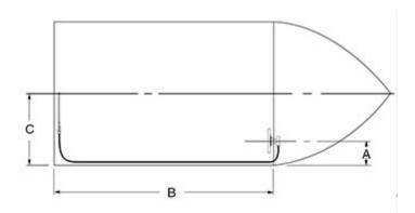
A single-cable, starboard drive push-pull mechanical cable system is shown in this diagram.
